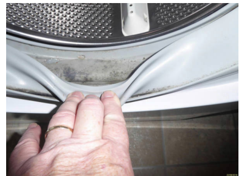
Inner seal stained
