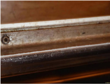
Dishwasher door edge stained/dirty
