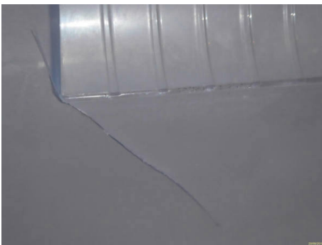
Crack base freezer drawer
