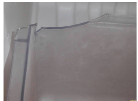
Crack base freezer drawer
