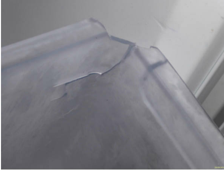
Crack base freezer drawer
